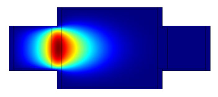
As the heater switches on, the gas around it warms up.
