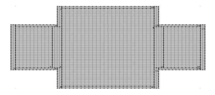
This is the mesh structure for the two-dimensional model used. Because it will be calculating a temperature *difference* of a few mK, it is essential that the mesh be symmetrical and the precision high. We refine the mesh until the calculated temperatures at symmetrically placed points agree to within a few µK.
