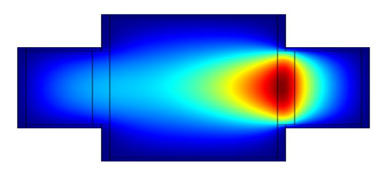
The cyclic temperature difference resulting from the diversion of the flow is too small to be seen from the colour plot, but we can record and graph it. The unusually high initial peak occurs as the gas first expands into a cold cavity.
